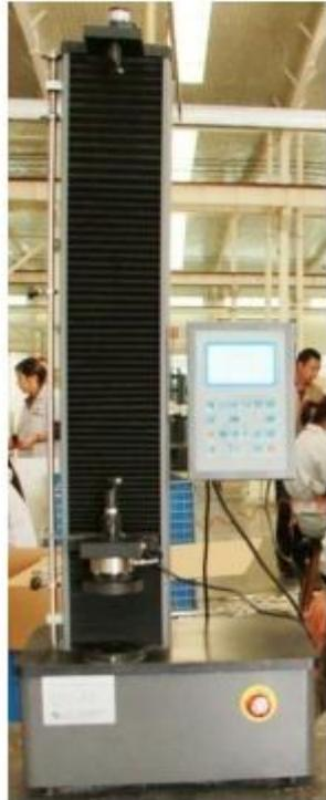
Automatic spring testing machine to test spring compression and tensile
