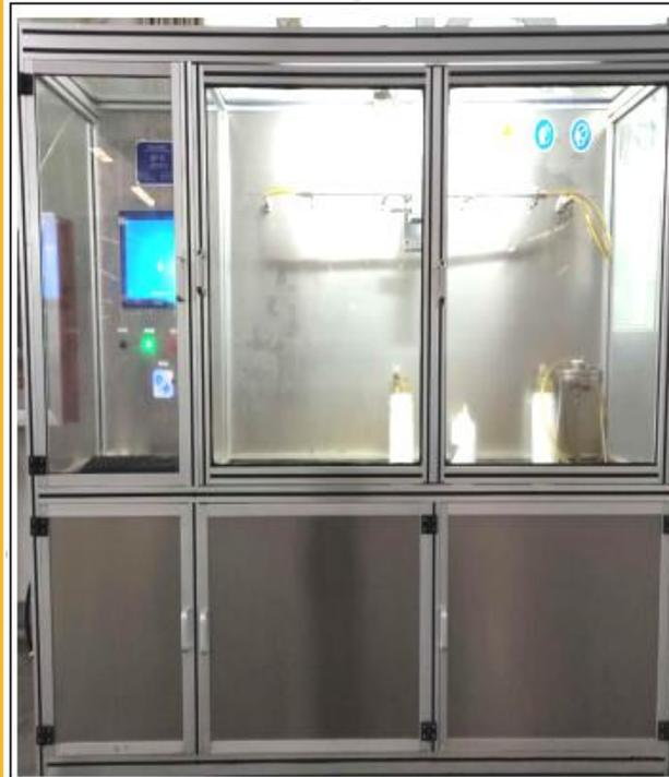
Fuel filter integrated test bench to test cleanliness and pressure drop flow characteristics.
