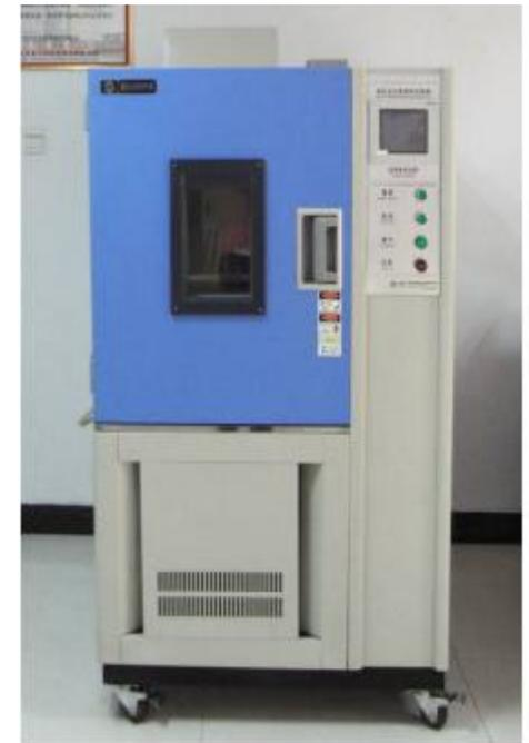
High and low temperature alternating humid heat test chamber to test the performance of filter and filter parts at high temperature 150°C or low temperature -40°C
