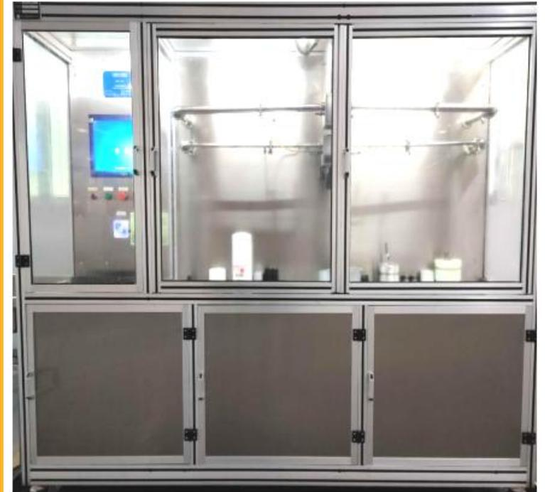
Flow resistance test bench to test filter rated flow resistance and bypass valve opening pressure.
