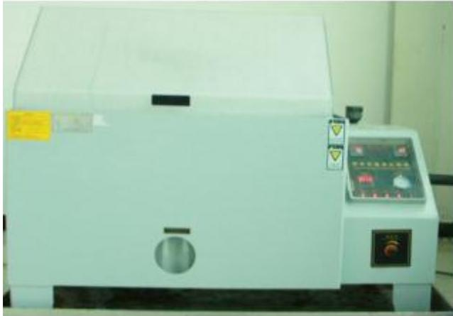
Salt spray corrosion test machine to test material corrosion resistance
