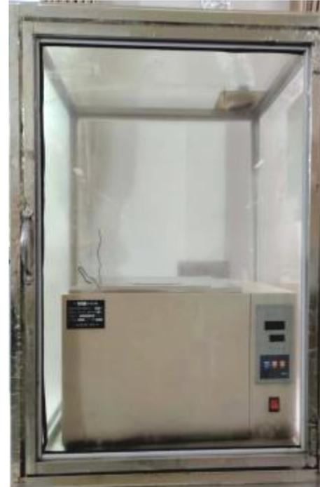
High oil temperature resistance test tank to test high oil temperature resistance of products and parts
