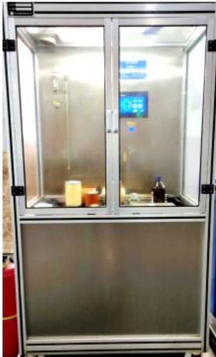
Bubble test bench to test the integrity of the oil filter element, and the maximum aperture and average aperture of the filter paper.
