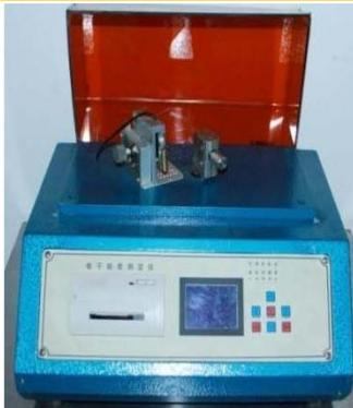
Electronic stiffness tester to test the tension generated by bending filter paper at a certain angle
