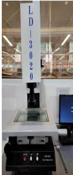
Quadratic image measuring Instrument to test rubber sizes
