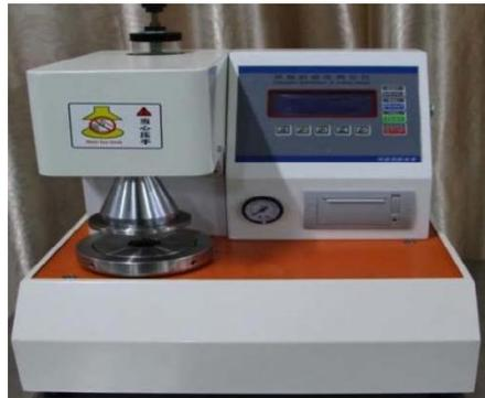
Paper breaking resistance tester to test the strength of filter media/ paper under pressure
