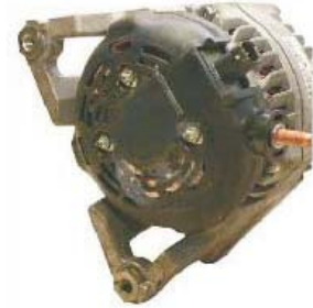
LESTER: 11298 OEM: 421000-0410 56028697AE DESCRIPTION: 160Amp/12Volt,CW,IR/IF, 7-Groove Pulley APPLICACION:
