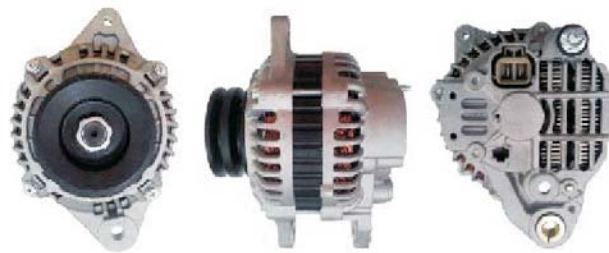
LESTER: 12637 OEM: A3T09699 DRA3473 4M40 DESCRIPTION: 90Amp/12Volt,CW,IR/IF, 2-Groove Pulley APPLICACION:
