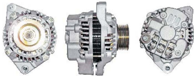
LESTER: 13820 OEM: 1-2232-01MI A2TB2991 DESCRIPTION: 75 Amp/12Volt, CW, IR /IF, 5-Groove Pulley APPLICACION: SUBARU FORESTER 1999-2002 H4 2.5L; SUBARU IMPREZA 1999-2001 H4 2.5L
