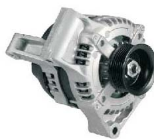
LESTER: 11035 OEM: 104210-3300 DESCRIPTION: 140Amp/12Volt,CW,IR/IF, 6-Groove Pulley APPILCATION:
