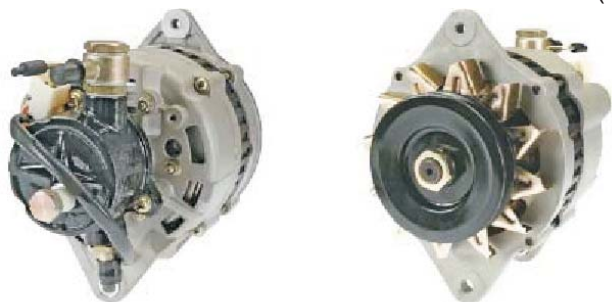
LESTER: 14613 OEM: 1-1121-01HI 23100-05E07 A3T35278 DRA3044 DESCRIPTION: 70Amp/12Volt,CW,IR/EF, 1-Groove Pulley APPLICATON: NISSAN Car &Lt Trk MAXIMA 2.8L(Diesel)1981-1983
