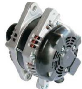
LESTER: 11323 OEM: 104210-2090 27060-31100 DESCRIPTION: 130Amp/12Volt,CW,IR/IF, 7-Groove Pulley APPLICACION:
