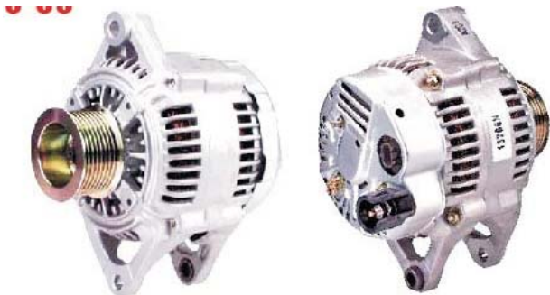
LESTER: 13766 OEM: 1-2227-01ND 121000-4280 DESCRIPTION: 136Amp/12Volt,CW,ER/IF, 8-Groove Pulley APPLICACION: DODGE RAM PICKUP 1999-2001 L6 5.9L
