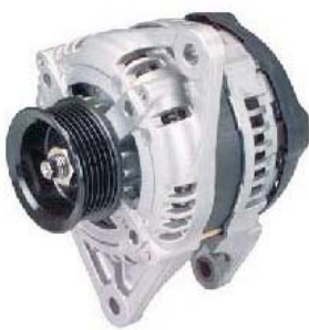
LESTER: 13923 OEM: 421000-0120 DESCRIPTION: 130Amp/12Volt,CW,ER/IF, 6-Groove Pulley APPILCATION:
