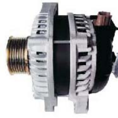
LESTER: OEM: 104210-5890 31100-R40-A01 DESCRIPTION: 130 Amp/12 Volt, CW, IR /IF, 7-Groove Pulley APPLICACION:
