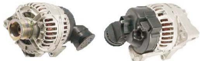
LESTER: 11045 OEM: 1-2599-01BO 0-124-415-035 DESCRIPTION: 105Amp/12Volt,CW,IR/IF, 6-Groove Pulley APPLICACION: BUICK REGAL 2004 V6 3.8L; CHEVROLET IMPALA 2004-05 V6 3.8L; CHEVROLET MONTE CARLO 2004-05 V6 3.8L
