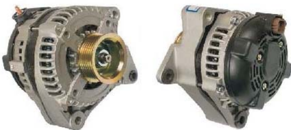
LESTER: 11090 OEM: 104210-3390 27060-0F050 DESCRIPTION: 150Amp/12Volt,CW,IR/IF, 6-Groove Pulley APPLICACION:
