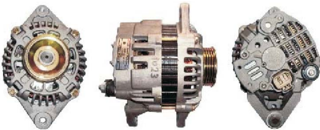
LESTER: OEM: KGP-221001017 OK-30D-18-300A DESCRIPTION: 90Amp/12Volt,CW,IR/IF, 4-Groove Pulley APPLICACION:
