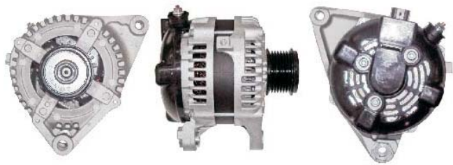
LESTER:11404 OEM: 27060-36040 DESCRIPTION: 130Amp/12 Volt, CW, IR /IF, 7-Groove Pulley APPLICACION:
