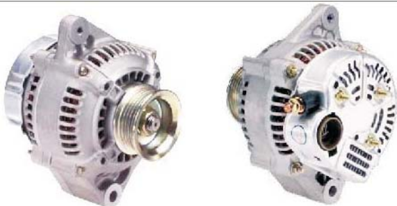
LESTER: 13240 OEM: 1-1039-01ND 100211-3352 27060-16122 DESCRIPTION: 70Amp/12Volt,CW,IR/IF, 5-Groove Pulley APPLICACION: GEO PRIZM 1989-92 L4 1.6L; TOYOTA CELICA 1990-93 L4 1.6L; TOYOTA COROLLA 1988-92 L4 1.6L
