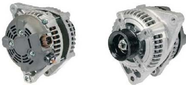
LESTER: 11033 OEM: 104210-3620 27060-OA120 9664219-362 DESCRIPTION: 130Amp/12Volt,CW,IR/IF, 6-Groove Pulley APPLICACION:
