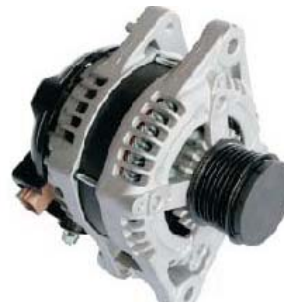
LESTER: 11323 OEM: 104210-2090 27060-31100 DESCRIPTION: 130Amp/12Volt,CW,IR/IF, 7-Groove Pulley APPLICACION:
