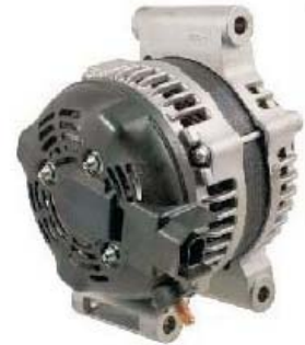
LESTER: 11140 OEM: 104210-4420 DESCRIPTION: 130 Amp/12 Volt, CW, IR /IF, 5-Groove Pulley APPILCATION:
