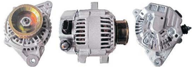
LESTER: 13755 OEM: 1-2086-01ND 101211-9600 27060-20040 DESCRIPTION: 90 Amp/12 Volt, CW, IR /IF, 6-Groove Pulley APPLICACION: TOYOTA CAMRY 1997-99 V6 3L
