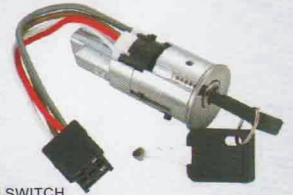
IGNITION SWITCH RENAULT R9 R18 013740/50 770057260
