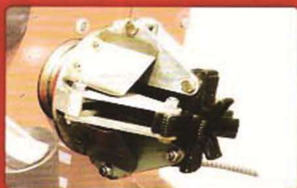
Clamping jaws are equipped with plastic protection to prevent ALU rims 特殊卡爪保护铝合金轮辋
