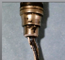
External oil contamination
