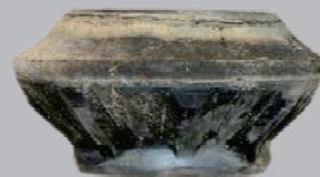
WORN RUBBER TOP SHOCK ABSORBER INFERIOR QUALITY
