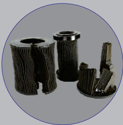
Yields to oil pressure result in deformation
