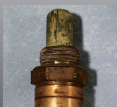
Ethylene Glycol (Antifreeze) Contamination
