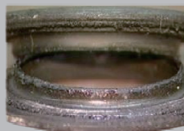
WORN SHOCK ABSORBER BEARING INFERIOR QUALITY
