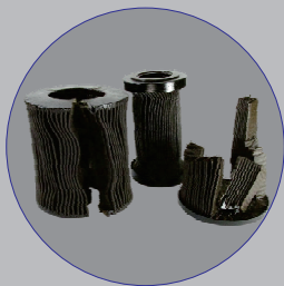
Yields to oil pressure result in deformation
